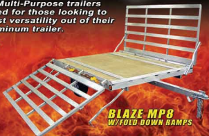
BLAZE MP SINGLE BELOW, W/OPTIONAL #12610 REAR RAMP KIT, #12760 FRONT RAIL KIT, & TONGUE JACK.
